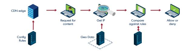
The way geo-fencing works is relatively simple. When a user request is made to the CDN edge, the IP address of the user's location is taken from the request header. A business-rules engine then compares that IP against a database of geo-locations. Based on that, the user's request for content is either approved or denied. If it's denied, the user can be presented with a webpage or message that indicates the content is not available in their area.
