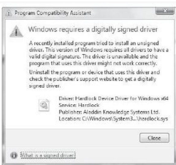
FIGURE 3-36 Warning when attempting to install an unsigned 64-bit driver
