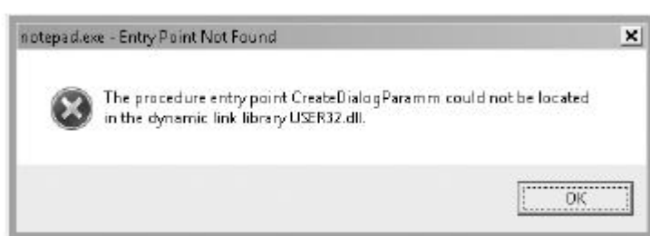
Figure 3-29 Dialog box shown when a required (imported) function is not present in a DLL
