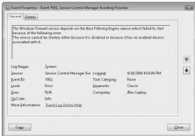
FIGURE 4-15 Service startup failure Event Log entry
