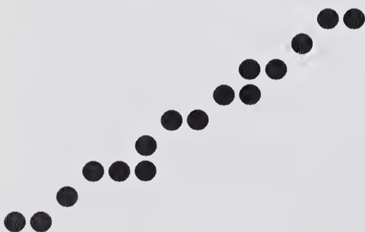
Figure 2-4 Output from a poor line-generating algorithm.
