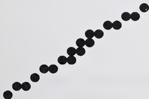
Figure 2-6 Uneven line density caused by bunching of dots.
