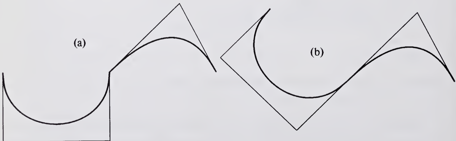
Figure 21-10 Continuity at joints between Bezier curves: (a) zero-order continuity; (b) first-order continuity.
