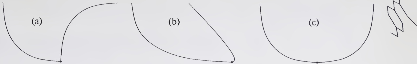
Figure 21-5 Orders of continuity at joints: (a) zero-order continuity; (b) first-order continuity (slope); (c) second-order continuity (curvature).
