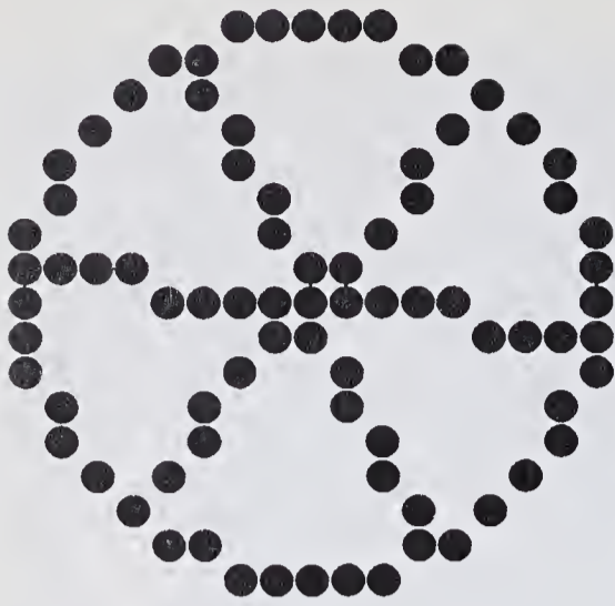
Figure 1-6 Raster image of a wheel, showing staircase-like quantization effects.
