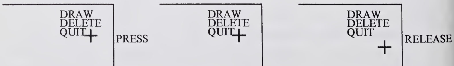
Figure 28-2 Aborting a menu command by moving the cursor away from the menu item. Note boldface selection feedback.
