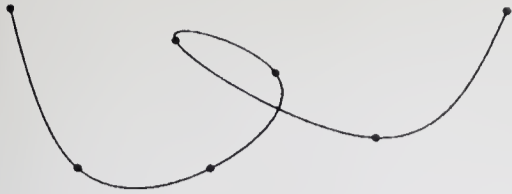
Figure 21-1 Control points (indicated by dots) govern the shape of a curve.
