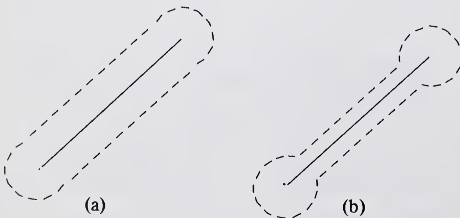
Figure 12-8 Gravity fields: (a) uniform, (b) with increased field strength at line endpoints.
