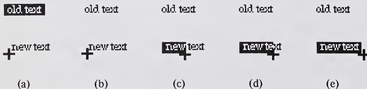
Figure 28-11 Text selection: (a) previous selection shown inverted; (b) on pressing down, old selection is removed; (c) and (d) as stylus moves, selection is shown inverted; (e) on releasing, selection remains inverted.
