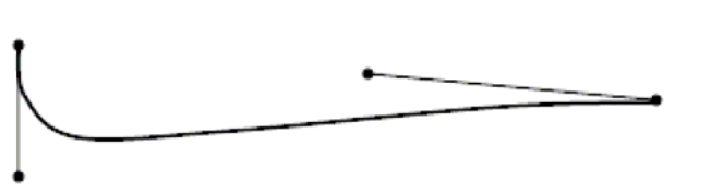
Figure 24(c) Reflex curves appear when you set the vectors in different directions
