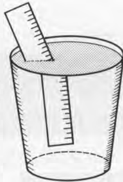
Fig. 9. Refraction causes the ruler to appear bent in a glass of water.
