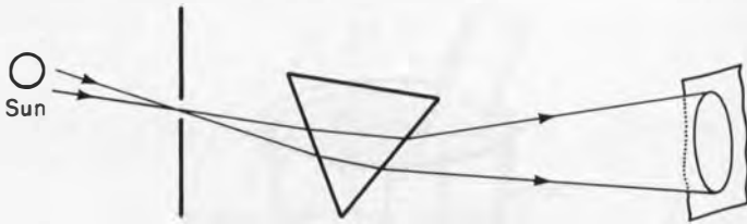
Fig. 11. Sunlight passes through the pinhole, strikes the prism, and is reflected to form a spectrum on a distant screen. Diagram adopted from Newton's Optiks , 1704.
